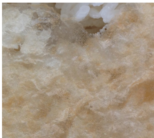
Figure C.5 – Example of Level 5 of burnt condition
