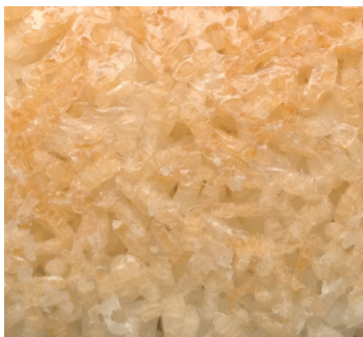
Figure C.9 – Example of Level 9 of burnt condition
