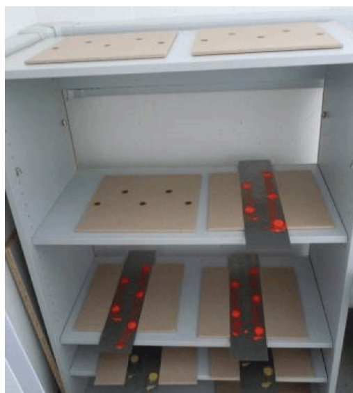
Figure 29 – Tile drying rack example
