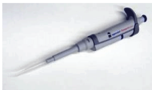
Figure 20 – Adjustable pipette 1 : 100 µl to 1000 µl range for applying liquid stains
