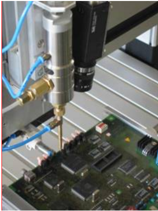
Fig. G10: Spraying a thick-film coating with Stream-Coat® (left) and assembly sprayed with thin-film protective coating (right)
