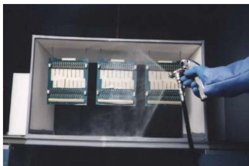
Fig. G2: Coating by spray process
