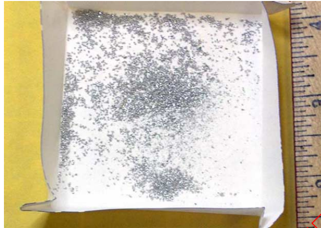
Figure 13 – Solder ball material collected from BGA using a hand removal procedure
