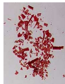
Figure 10c – IC package after disjointment
