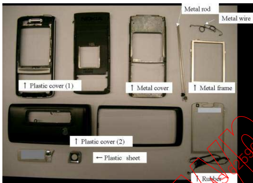
Figure 7 – Complete disassembly of the other housing/frame
