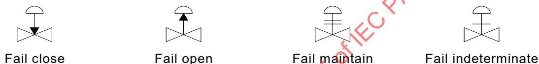
Figure B.33 – Signal failure valve action
