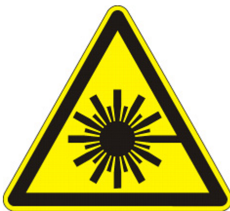
Figure 3 – Warning; Laser beam symbol (ISO 7010-W004:2011-05),
