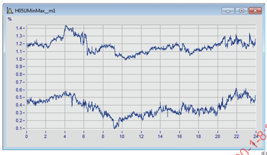
Figure 25 – Minimum-maximum envelope curves of the 5 th harmonic voltage level at test site M1
