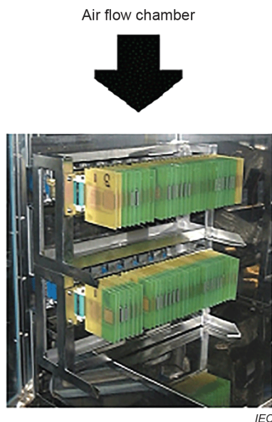
Figure 3 – Sample orientation in test chamber
