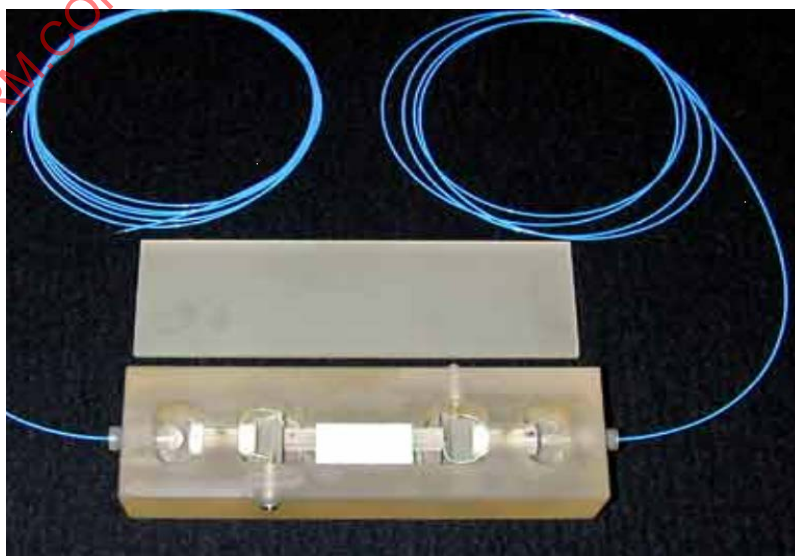
Figure 30 – Industrial bulk Pockels Cell (courtesy of Alstom Grid)
