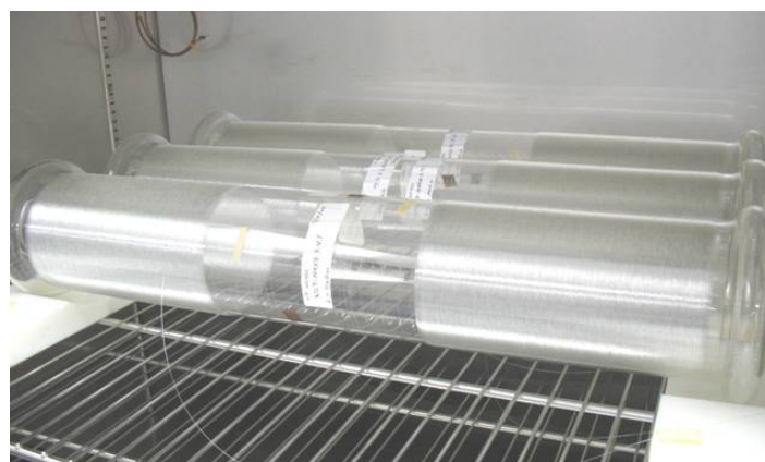
Figure 7 – Basketweave example as used in an optical fibre testing facility
