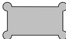
Figure 11 – Corner relief in the cavity of a chip tray
