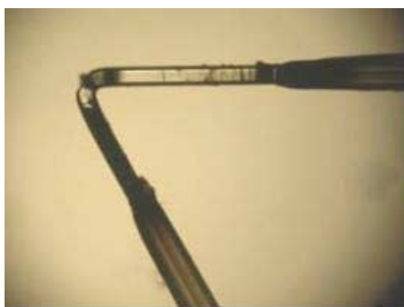
Figure A.3 – Typical R1 failure characteristics with a loss of greater than 10 dB
