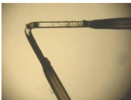
Figure A.3 – Typical R1 failure characteristics with a loss of greater than 10 dB
