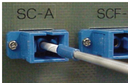
Figure 11 – Cleaning ports using a stick type cleaner
