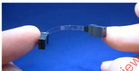
Figure 6c- Flexible optical circuit board using optical waveguides
