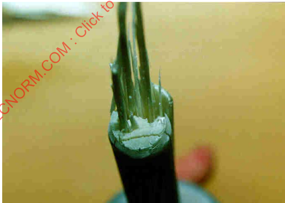
Figure 1 – Typical brittle fracture
