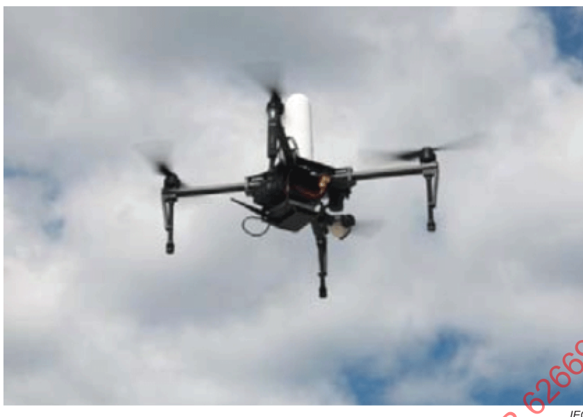
Figure 11 – Drone used for field measurements around the BS site
