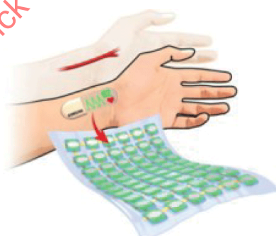
Figure 7 – Example of stretchable display for wearable application [3]
