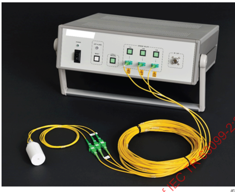
Figure 3 – 3-axis electric-field sensing system using LN optical modulator
