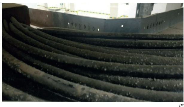
Figure 3 – Fungal growth on optical cable with TPU sheath
