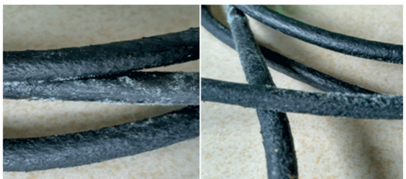
Figure 1 – Fungal growth on optical cable with PVC sheath
