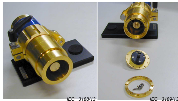
Figure 75 – Detailed views of the contact area the test fixture and the secondary side of side opened
