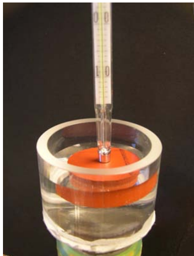
Figure C.1 – Example of a measurement set-up to measure the temperature rise due to ultrasound in absorbing material
