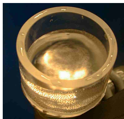
Figure 1 – Several examples of how to prepare a set-up to check the distortion on the water surface due to ultrasound
