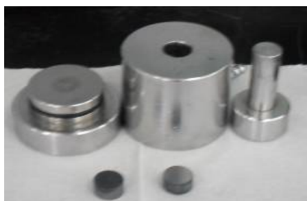
Figure 1 – Appearance of die for compacted density measurement
