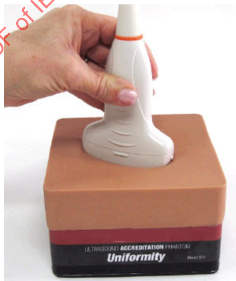
Figure A.4 – A compact uniformity phantom of relatively durable rubber material
