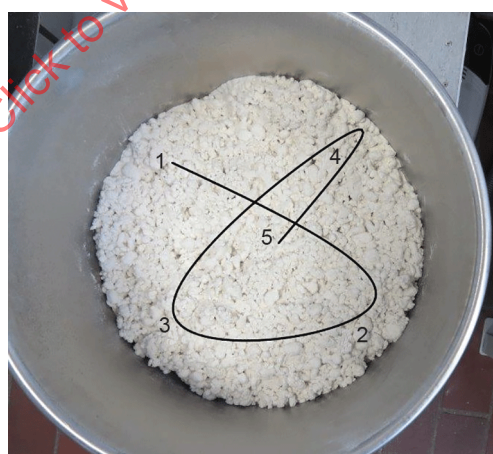
Figure 4 – Order of sampling (star-shaped)
