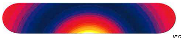
Figure E.8 – Current density in the central cross section of the hand model at 9 mm from the wire – Flux® 12 FEM modelling
