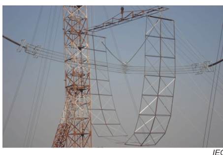
Figure B.3 – 1 200 kV air-gap experimental tests
