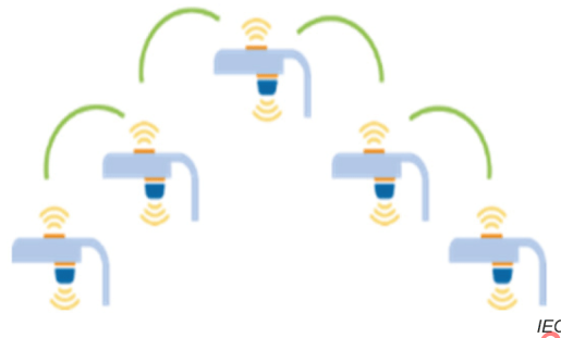
Figure 3 – Example of autonomous lighting system
