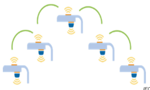
Figure 3 – Example of autonomous lighting system
