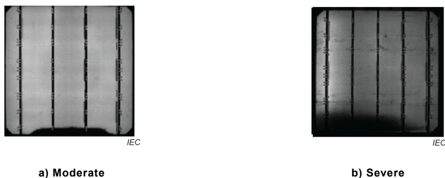
Figure 5 – EL images of PV cell with local shunting
