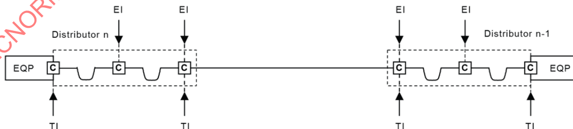
Cabling subsystems 2, 3 and 4
