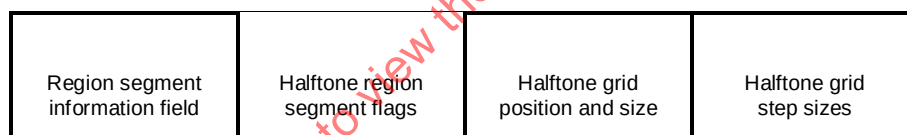
Figure 41 – Halftone region segment data header structure
