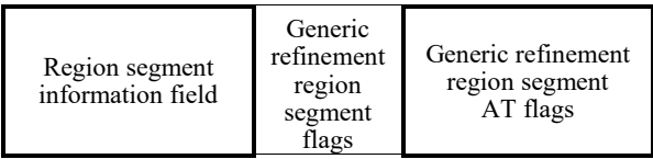
Figure 52 – Generic refinement region segment data header structure
