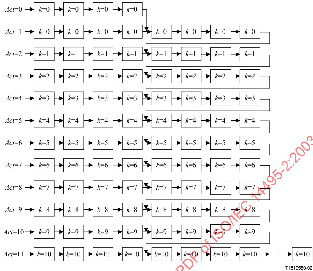
Figure A.19 – Binary decision tree for lossless coding with qbpp ≥ 10
