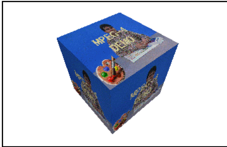
Figure 14 — A CompositeTexture2D example. The 2D scene is projected onto the 3D cube.
