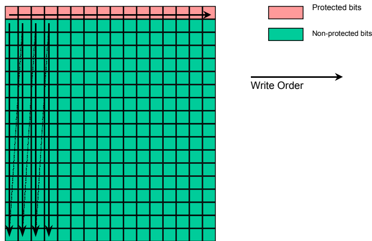
Figure 1.12 – One stage of interleaving
