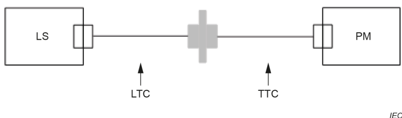
Figure 18 – Connection of LTC to TTC to verify attenuation of reference connectors
