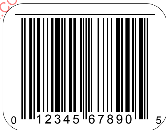
Figure C.1 — Line for detecting print head element burnout
