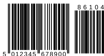
Figure 6: EAN-13 bar code symbol with 5-digit add-on
