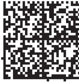
Figure A.3 — Test symbol for Fixed Pattern Damage (Data Matrix)
