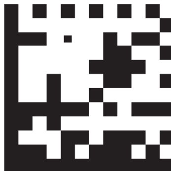
Figure A.1 — Example test symbol for Modulation
