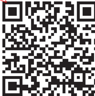
Figure A.4 — QR Code symbol with Fixed Pattern Damage
