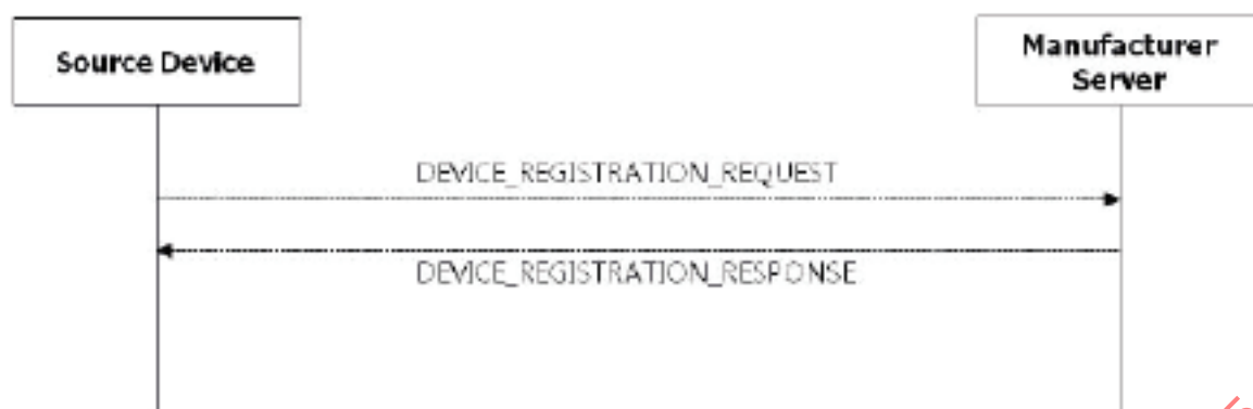
Figure 12 — Device Registration Operation
