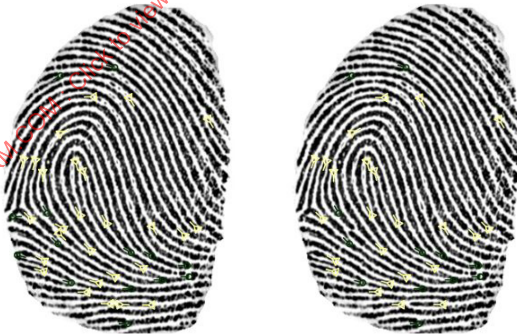
Figure E.3 — Liberal minutia detection (left) versus conservative minutia detection (right)
