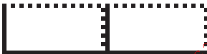
Figure C.1 — Alignment bar configuration for 12 \times 48 rectangular symbol
