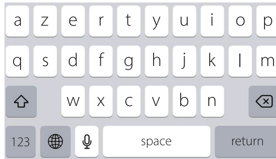
Figure 5 — Example of a mapping of an AZERTY keyboard layout on a French on-screen keyboard
