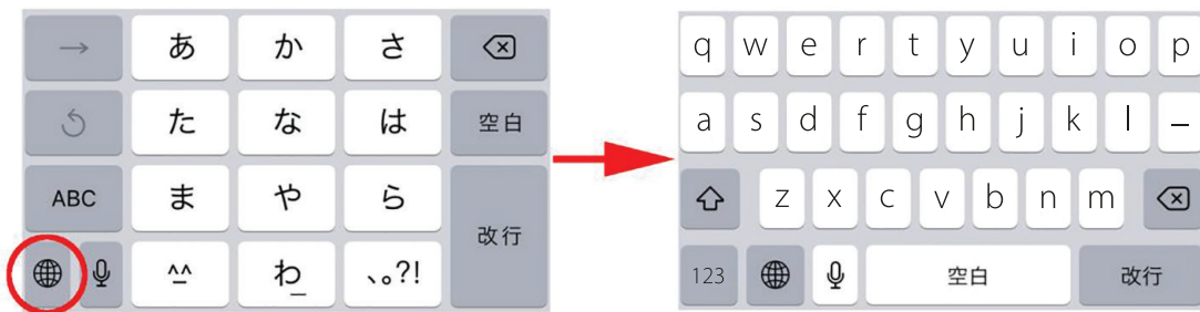
Figure 9 — Example of a language selection key with an on-screen keyboard
