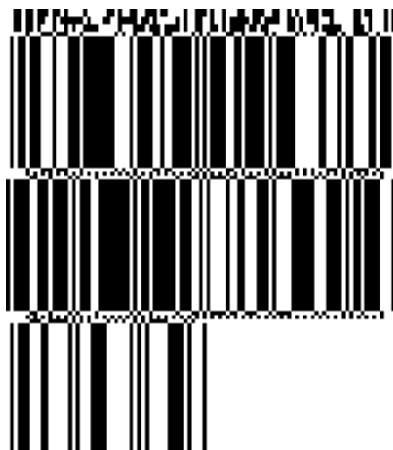
Figure 10 — A GS1 DataBar Expanded Stacked Composite symbol (with CC-A), encoding 010001234567890510ABCDEF and 2112345678 respectively
