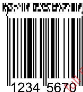
Figure 4 — An EAN-8 Composite symbol (with CC-A), encoding 12345670 and 21A12345678 respectively
