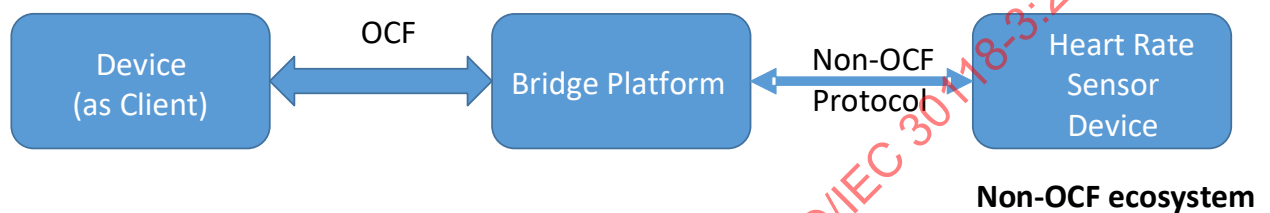
Figure 1 – Server bridging to Non-OCF device
