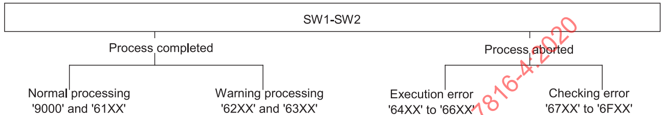
Figure 2 — Structural scheme of values of SW1-SW2
