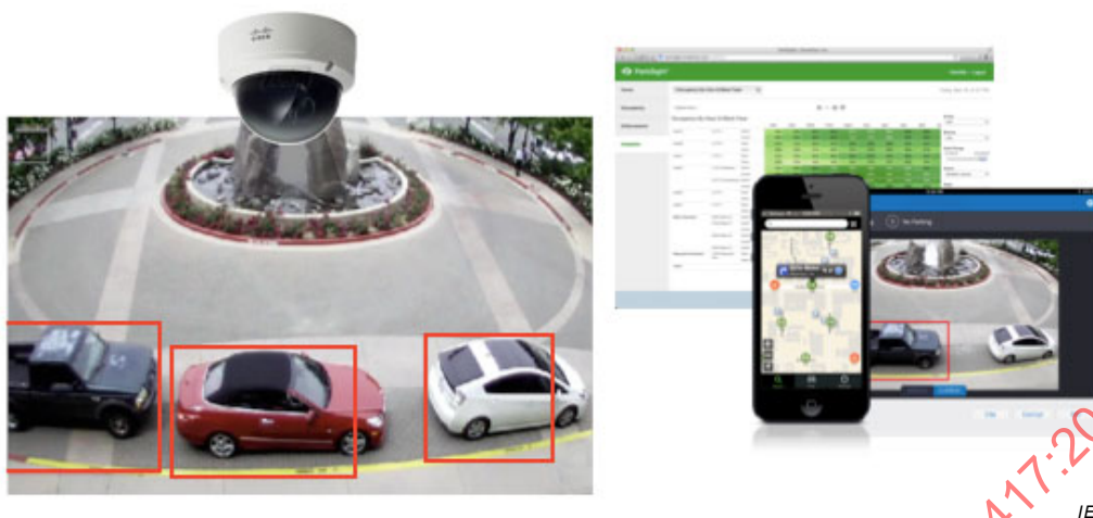
Figure 26 – Camera based identification of traffic load at key points in the infrastructure
