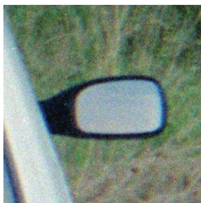
a) 4000 dots per inch (2.54 cm) scan of 2 mm × 2 mm area
