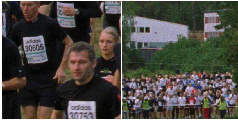
Figure 3 — Kodak Vision™ 2) 250D film and 3063 dots per inch (2.54 cm) scan of 2.7×2.7 mm areas of the same picture
